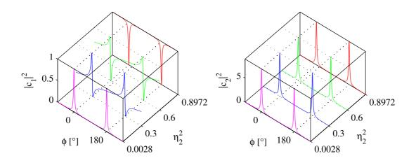
**Figure 3.** left: Power reflectance  $|c_1|^2$  of cavity back reflecting port for a grating cavity with end mirror reflectivity  $\rho_1 = 1$  and cavity coupling  $\eta_1^2 = 0.1$  for selected values of  $\eta_2$ ; right: power inside the cavity  $|c_2|^2$ .
