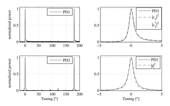
Figure 6. Normalized Measured power at PD1 and PD2 and corresponding theoretical curves.
