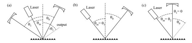
**Figure 1.** (a) grating in non Littrow configuration with two existing orders can be used as a beam splitter for a Michelson interferometer; (b) linear grating Fabry-Perot interferometer in 1st order Littrow mount; (c) 2nd order Littrow mount.
