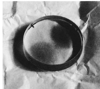
FIGURE 5. Left: Schematic view of one glass sample to be radiated in four different spots with different dose. Right: Sample showing the strongest darkening in the spot radiated with 200 krad.
