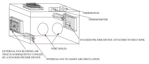
Figure 2. Temperature controlled environment used to fabricate silicate bonds at various temperatures below room temperature.
