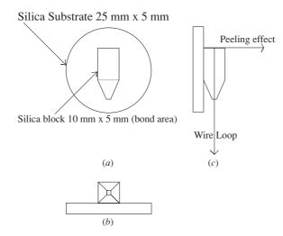
**Figure 4.** Example of a silica to silica bond used for strength testing: a wire loop is placed around the silica block and attached to a linear drive to test the mechanical strength of the bond. The line of action of the wire is offset from the bond line thus creating a peeling effect at the top edge of the silica block as shown in (c).
