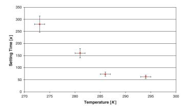
Figure 3. The dependance of settling time with temperature using a sodium hydroxide bonding solution (molecular ratio 1:256 NaOH:H<sub>2</sub>O) for silica to silica bonds of bond area  $\approx$ 50 mm<sup>2</sup>.
