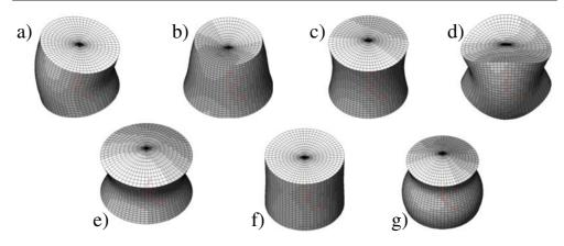
**Figure 4.** Shapes of the detected modes. (a) Bending, (b) first asymmetric, (c) fundamental, (d) clover, (e) symmetric, (f) expansion, (g) second asymmetric.
