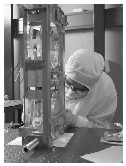
Figure 1. Intermediate mass on top and mirror at the bottom clamped in a steel frame. On the first plane the ears are bonded on both the masses and the two fibres welded.
