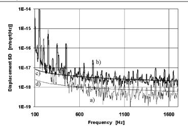
**Figure 3.** Displacement spectral densities. Curves (a) and (b) are recorded from the interferometer output before and after putting grease on one of the masses, respectively. Curves (c) and (d) are estimations using a Q of 1800 for the greased mass and  $1.2 \times 10^5$  for the others.
