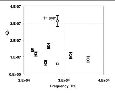
**Figure 5.** This plot shows the comparison between the measured loss factor for each mode (circles) and the estimated loss factor (squares) as they come from a three-parameter linear fitting. The symmetric mode data were removed from the fitting process because they show a significantly higher loss than the estimated one.
