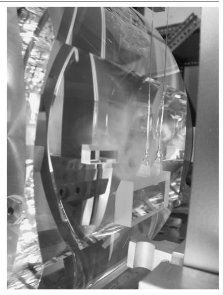
Figure 2. Detail of two fibres welded on the tips of a mirror ear.
