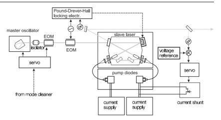
Figure 1. Scheme of the GEO 600 injection-locked laser system.
