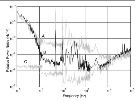
**Figure 3.** Relative power noise spectral density of the laser system: (A) without stabilization circuit, (B) out-of-loop signal with independent photoreceiver (not displayed in figure 1) and (C) upper limit of the in-loop signal. Below 10<sup>3</sup> Hz the true in-loop signal is covered by the spectrum analyser input noise.
