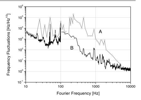
**Figure 2.** Spectral density of the eigenfrequency fluctuations of the slave laser cavity. The data are derived from the piezo length actuator signal that is necessary to keep the slave laser exactly in resonance with a frequency-stabilized master oscillator. (A) Conventional laser resonator assembled from multiple discrete components. (B) Quasi-monolithic slave laser resonator.
