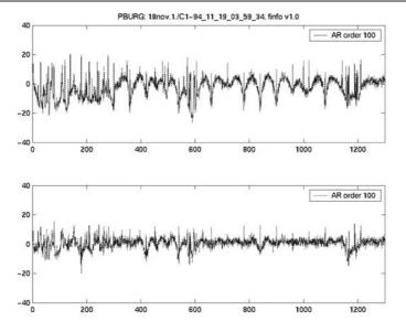
**Figure 3.** Caltech 40 m 1994 data run: each plot shows the ratio of PSD (IFO\_DMRO channel) obtained from Welch's method to that obtained from an AR(100) model: (top) without line removal and (bottom) with line removal.
