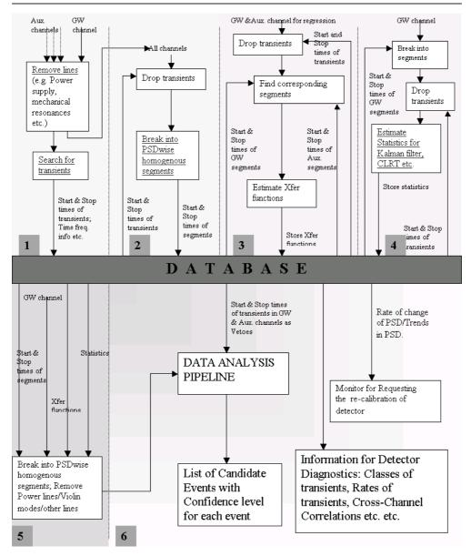
Figure 1. A schematic diagram of the DCR algorithm.
