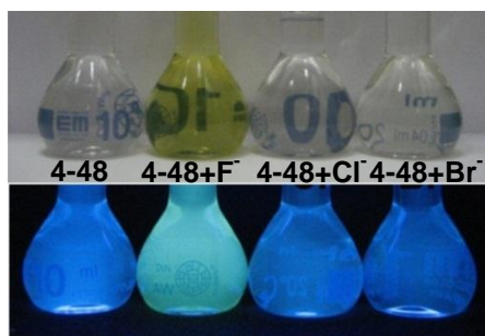
Figure 4-63: Colorimetric response of macrocycle 4-48 ( c = 10^{-5} M in THF) to fluoride (10 eq) anion under ambient light and \lambda = 366 nm.
