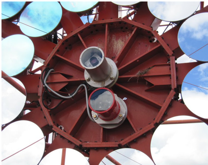
Figure 4.2.: The picture shows the LidCCD in the central part of the CT2 dish and the SingleCCD in the bottom right part.
