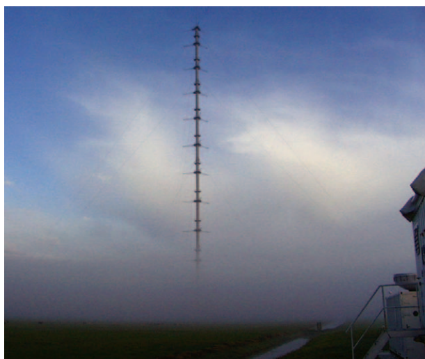
FIG. 2. The 213-m tower at the Cabauw site in the Netherlands, with its base partially obscured by morning fog. The 35-GHz cloud radar can be seen on the right. (Figure courtesy of Jacques Warmer.)
