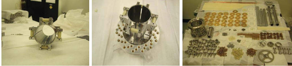
Figure 6.13: Left and Middle: Pictures of the four-split cylindrical steerer in the magnetic fringe field of the magnet. The middle picture shows the close location to the feed-through section. The picture on the right displays many of the fabricated parts for the CPET trap structure.
