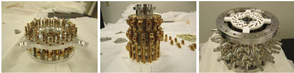
Figure 6.14: Pictures of the CPET feed-through section. The left picture shows the feed-through plugs that are part of the trap structure. The middle picture displays an intermediate stage of the assembly, whereas the right picture is the complete feed-through section.
