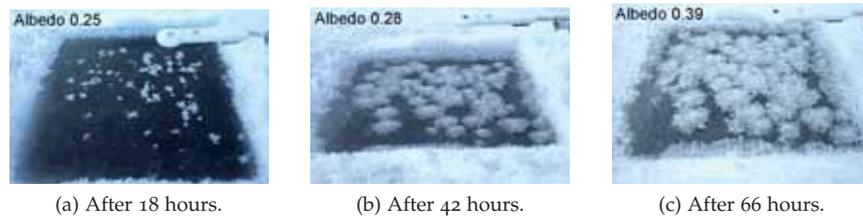
Figure 2.3: Evolution of the frost-flower coverage of the sampling hole besides the hole with thermistor rods from 17 March until 20 March.
