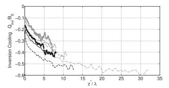
FIG. 7. Rate of change of buoyancy at the inversion as a function of the convective boundary layer length scale. The color codes the Richardson number: black for  $Ri_0=57$  and gray for  $Ri_0=10$ . The type of line codes the Reynolds number: points over lines for  $Re_0=1600$ , solid for  $Re_0=800$ , dashed for  $Re_0=400$ , and dashed–dotted for  $Re_0=90$ .
