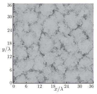
FIG. 3. Horizontal cross section of the smoke field. The color scale ranges from s=0.4 (black) to s=1.0 (white). The section was extracted from a horizontal cut one optical length below the inversion ( $z=z_i-\lambda$ ). The parameters of the simulation are (Ri<sub>0</sub> = 10, Re<sub>0</sub> = 800).
