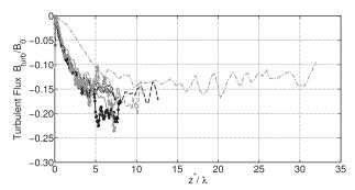
FIG. 8. Turbulent exchange of energy at the inversion point as a function of the convective boundary layer length scale. The color codes the Richardson number: black for  $Ri_0=57$  and gray for  $Ri_0=10$ . The type of line codes the Reynolds number: points over lines for  $Re_0=1600$ , solid for  $Re_0=800$ , dashed for  $Re_0=400$ , and dashed–dotted for  $Re_0=90$ .
