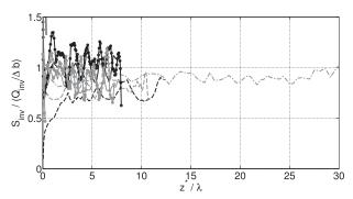
FIG. 11. Flux of noncloudy air into the cloud divided by the change of buoyancy in the cloud. The color codes the Richardson number: black for  $Ri_0 = 57$  and gray for  $Ri_0 = 10$ . The type of line codes the Reynolds number: points over lines for  $Re_0 = 1600$ , solid for  $Re_0 = 800$ , dashed for  $Re_0 = 400$ , and dashed–dotted for  $Re_0 = 90$ .
