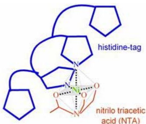
Figure 4-1: Schematic representation of how two histidines from a poly-histidine-tag interact with Ni-NTA taken from http://www.biologie.uni-osnabrueck.de/Biophysik/Piehler/grafik/research_figure4new.jpg
