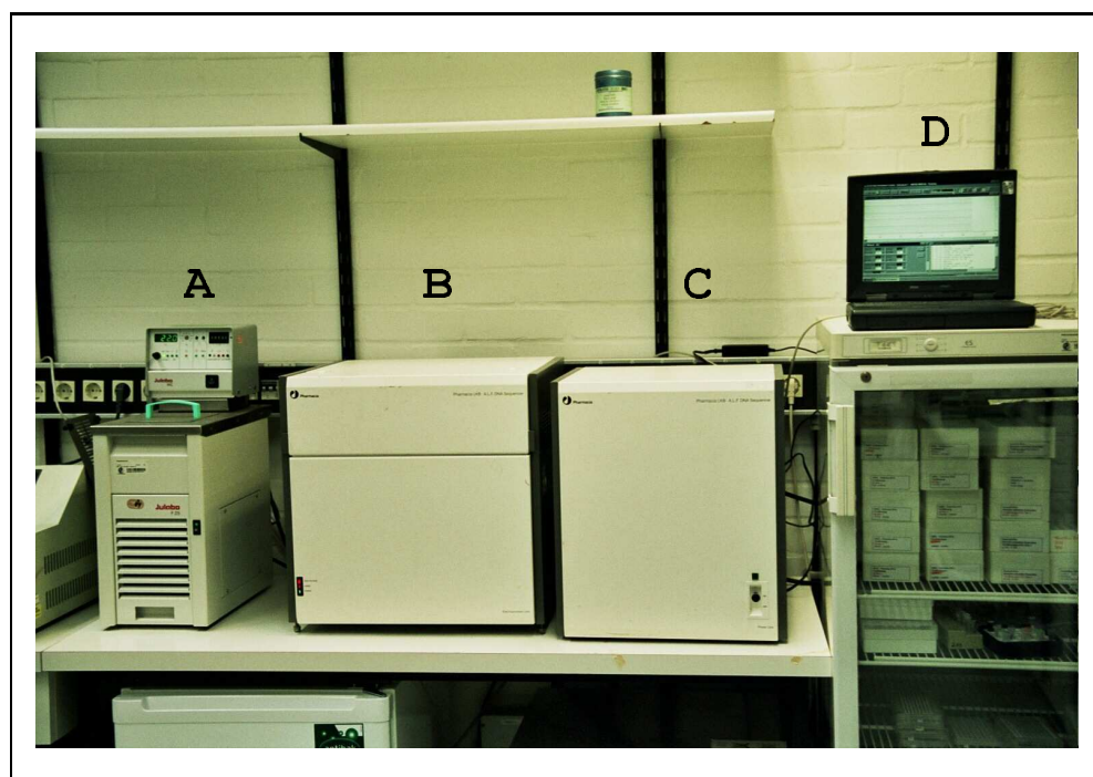
Figure 14: Components of the A.L.F. EMSA System. The system consists of a power supply (C) that drives an electrophoresis unit (B). The temperature of the polyacrylamide gel in the electrophoresis unit can be increased by the device itself, but cannot be decreased to room temperature or lower, so that an external thermostat (A) had to be used to prevent thermal denaturation of the proteins during electrophoresis. All parameters of the run were adjusted in the ALFWin software on a notebook (D), despite the temperature of the external water circulation which was directly set at the thermostat.
