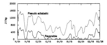
Figure 4. Time variations of convective available potential energy (J kg<sup>-1</sup>, 5-day running mean) over the intensive flux array during the TOGA-COARE intensive observing period. The solid and dashed lines represent air parcels originating from 1000 hPa undergoing reversible and pseudo adiabatic processes, respectively; ice effects are not considered. See Lin and Johnson (1996) for a discussion of data and analysis methods.
