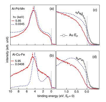
FIG. 1 (color online). HAXPES valence band spectra measured with  $h\nu = 5.95$  keV at 300 K compared with surface sensitive low energy photoemission spectra from the literature [7,9] for (a) *i*-Al-Pd-Mn and (b) *i*-Al-Cu-Fe. The spectra have been normalized to the same intensity at the Pd 4*d* and Cu 3*d* main peak for Al-Pd-Mn and Al-Cu-Fe, respectively. The near- $E_F$  region is shown along with the Au Fermi edge (black open circles) for (c) Al-Pd-Mn and (d) Al-Cu-Fe.
