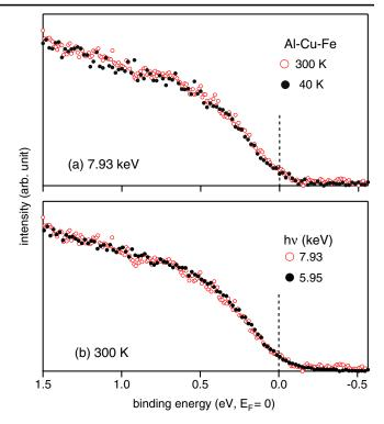
FIG. 3 (color online). The near- $E_F$  region of the HAXPES valence band spectra of Al-Cu-Fe measured with (a) 7.93 keV photon energy at 40 K and 300 K and (b) 7.93 and 5.95 keV photon energies at 300 K.
