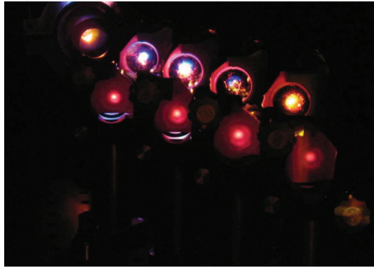
Figure 2.8: Customized chirped-mirror compressor placed after the hollow fiber.
