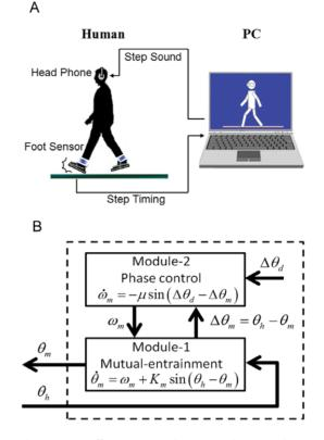
**Figure 1. WalkMate overview.** A) Schematic depiction of the WalkMate system. B) The computer's timing system used nonlinear oscillators and was organized hierarchically in two modules. Module 1 mutually entrained the gait frequencies of the computer and the participant. Module 2 adjusted the relative phase difference between the computer's auditory onset and the participant's step contact to a target phase difference [more details in the Materials and Methods section].
