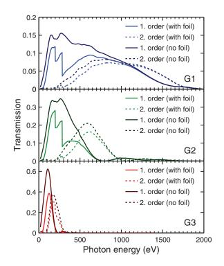
FIG. 3. Calculated photon energy dependence of the combined transmission of the gratings and the C-parylene foil (thickness 234.5 nm). Grating efficiencies were calculated using the REFLEC program.<sup>31–33</sup> Data for the transmission of the foil were taken from Ref. 34. Darker curves show transmission without the foil (only grating efficiency).
