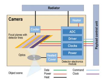
FIG. S3. MSI. (top) Instrument concept. (bottom) Top-level architecture for its cameras.
