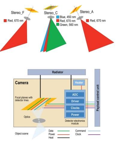
Fig. S2. MAI. (top) Instrument concept. (bottom) Top-level architecture for its cameras. ADC is analog-to-digital converter.
