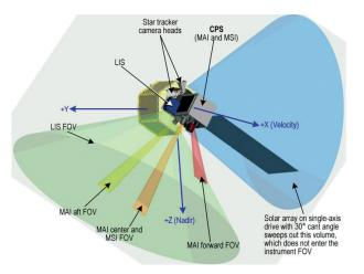
FIG. SI. The CHASER spacecraft uses high-heritage components, resulting in a low-risk mission.
