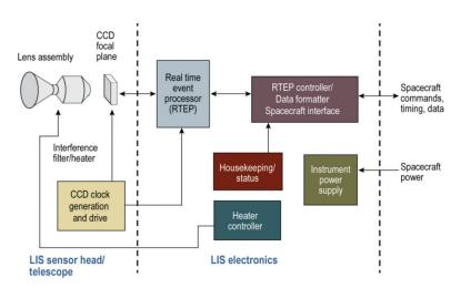
FIG. S4. LIS Functional block diagram. CCD is charge-coupled device.
