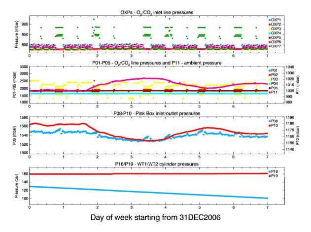
Fig. 2. Example of diagnostic parameters, showing all pressures relevant to the  $O_2$  and  $CO_2$  system over a one-week period starting from 31 December 2006. Each data point in the figure is a 16 min average (for all parameters). The labels in the legends correspond with those shown in Fig. 1.
