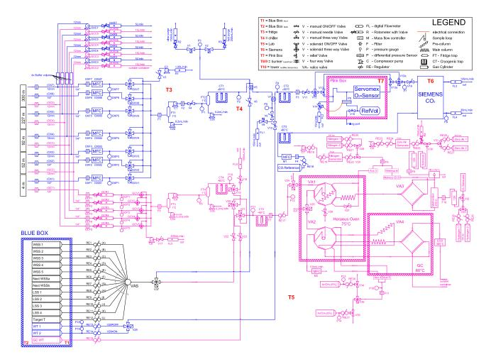
Fig. 1. Gas-handling schematic for atmospheric measurements of  $O_2$  and  $CO_2$  (shown in blue), and  $CH_4$ , CO and  $N_2O$  (shown in pink). As schematically represented, there appear to be dead volumes downstream of 3-way valves OXV1-7 and GCV1-5, however, in reality they are mounted in a manifold arrangement with zero dead volume.
