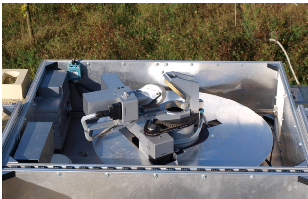
Fig. 3. The Bruker Solar Tracker type A547 mounted in the custom made dome (shown in open state).
