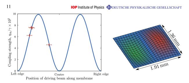
**Figure 4.** (a) The coupling parameters that fit the four datasets are consistent with the excitation of the (2, 1) mode of the membrane (shown in (b)); the solid curve represents the sinusoidal profile of the squared amplitude of this mode. (b) Vibrational profile of the (2, 1) mode of the membrane.
