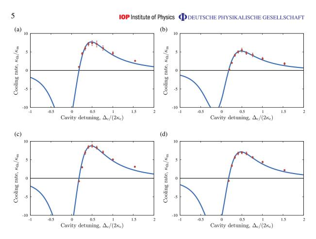
**Figure 3.** Fits to four sets of experimental data; dataset 1 is the set reported in [13]. The four sets of data differed in the location of the driving beam on the membrane and in the driving wavelength  $\lambda_L$  used. All other system parameters are reported in the text and in table 1. (a) Dataset 1;  $\lambda_L = 870$  nm; (b) dataset 2;  $\lambda_L = 852$  nm; (c) dataset 3;  $\lambda_L = 852$  nm; (d) dataset 4;  $\lambda_L = 852$  nm.
