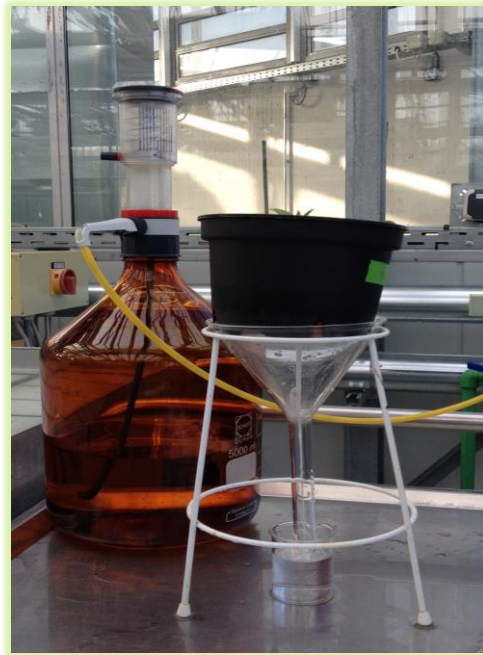
Figure 5. Setup for the collection of RE. The pot was placed on top of a glass funnel and with a 25 mL dispenser tap water was distributed over the sand. RE were collected in a 50 mL beaker and transferred to 50 mL falcon tubes.
