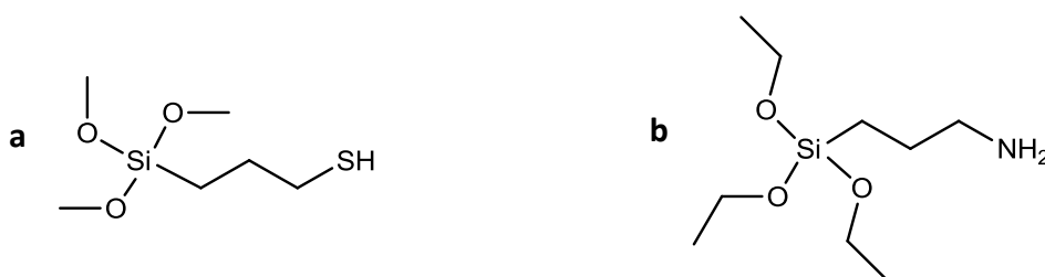
Figure 5.7 Chemical structures of ( a ) 3-mercaptopropyltrimethoxysilane (MPTMS) and ( b ) 3-aminopropyltriethoxysilane (APTES).
