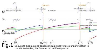
Methods: The slab-selective, BOLD-corrected pulse sequence was implemented on a Siemens 7T MRI scanner. Fig.1 shows the sequence diagram and corresponding spin magnetization. The study was approved by the local ethics committee and all subjects gave informed consent. The scan parameters were: voxel size = 1.5 mm isotropic, TE/TI/TR=19/1330/1500ms. We acquired data with 2D multi-slice single-shot GRE EPI without slice gaps. We implemented a tr-FOCI pulse [6] to achieve
