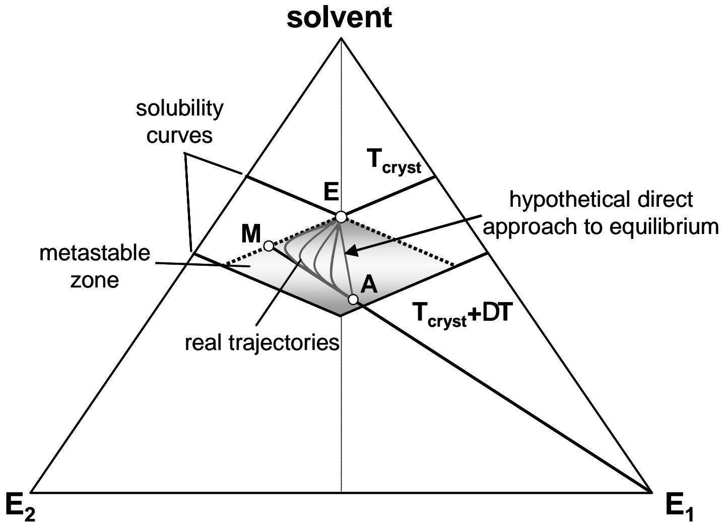
**Fig. 1:** Principle of preferential crystallisation illustrated in ternary phase diagram.
