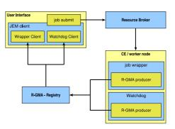
Figure 3: Job Execution Monitor, global principle
