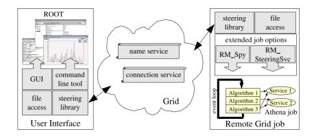
Figure 5: The components of RMOST
