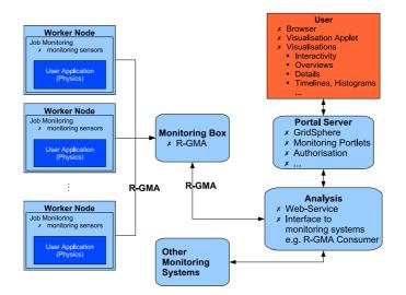
Figure 2: Architecture of the Job and Resource Usage Monitoring System
