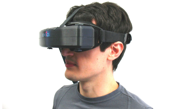
Figure 3.1: Sensics xSight 6123 HMD. The HMD is mounted on the head with three adjustable strips that meet at the back of the head where a knob can be used to adjust the tension.
