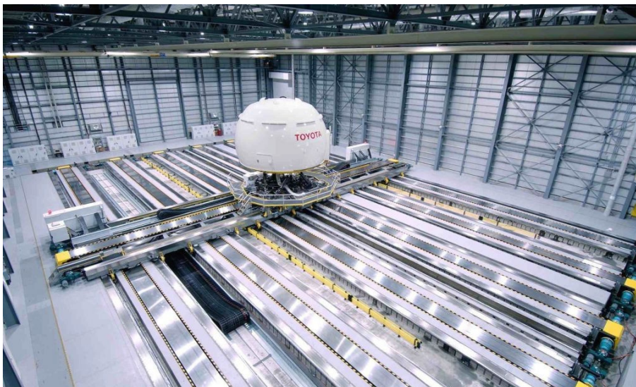
Figure 1.13: Toyota's driving simulator. The dome with a mock-up car inside is mounted on a hexapod which itself is located on a two dimensional cartesian platform. Picture taken from [Toyota Motor Corporation, 2010].
