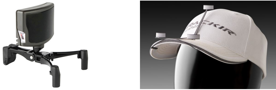
Figure 2.6: Head tracking system ‘Track IR 5’ from Naturalpoint. (a) The ‘Track IR 5’. An infrared camera with four powerful infrared LEDs at its side is located behind the black window. LEDs on the side indicate the status of the system. (b) Reflective clip attached to a base ball cap. The system tracks the three reflective markers and calculates orientation and position from their relative position to each other. Pictures taken from [NaturalPoint Inc., 2010]
