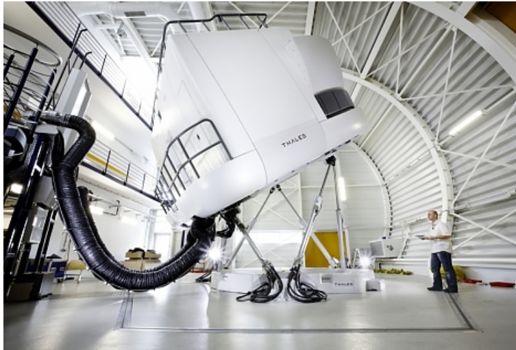
Figure 1.12: Lufthansa's A380 motion simulator at Frankfurt Airport. A mass of 15 t is moved through a hexapod platform. Picture taken from www.lufthansa.de .
