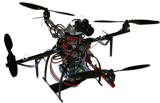
Fig. 2: The UAV used in our experiments instrumented with reflective markers to be tracked by our Vicon system
