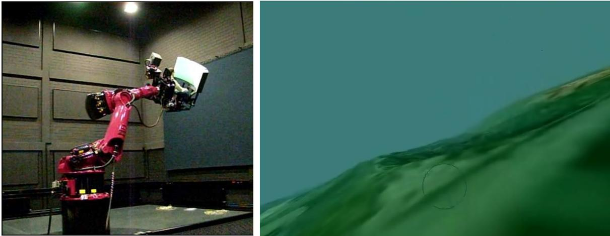
Figure 5. The MPI Motion Simulator and a snapshot of the graphical environment.
