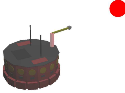
Figure 5.5: Observation with image moments. The camera is mounted on the end-effector of a NMM in a typical eye-in-hand configuration. The red sphere represents the target object tracked during the simulation.
