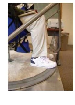
Biomechanical vection stimulus: Blindfolded participants were sitting on a stachair hammock tionary mounted above a circular treadmill that rotated at 60°/s, and were stepping to compensate for the floor's rotation.
