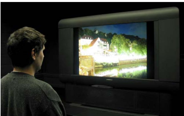
Figure 1. Brightside DR37-P HDR display. This display has a resolution of 1920x1080 pixels and a contrast ratio of 200,000:1. It is able to simultaneously show both dark and very bright pixels. www.brightsidetech.com
