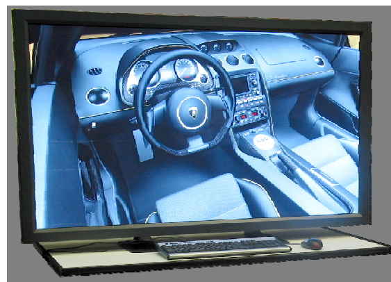
Figure 2. EYE-LCD5600DHD. This display has a resolution of 3840x2160 pixels and a panel size of 1224x729 mm (56" diagonal). www.eyevis.de
