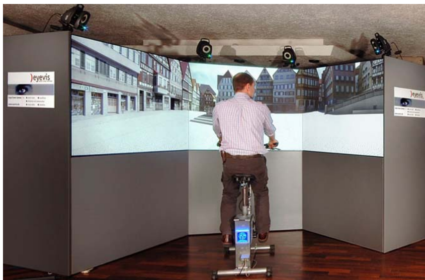
Figure 4. Multipanel tiled display based on 67" SXGAplus back-projection cubes (eyevis ImmersiveCUBE system).
