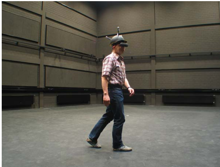
Figure 8. User wearing an HMD and a tracking helmet for navigation in large VEs (setup at the Cyberneum ( www.cyberneum.de ) of the Max Planck Institute for Biological Cybernetics).
