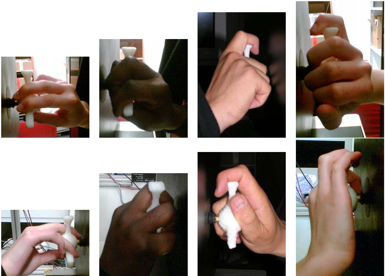
Fig. 8. Experiment 2: Variation in number of tips contacted while gripping. From left to right: 0, 1, 2, and 3 object tips contacted. Top and bottom rows show different viewpoints of same subject's grip.
