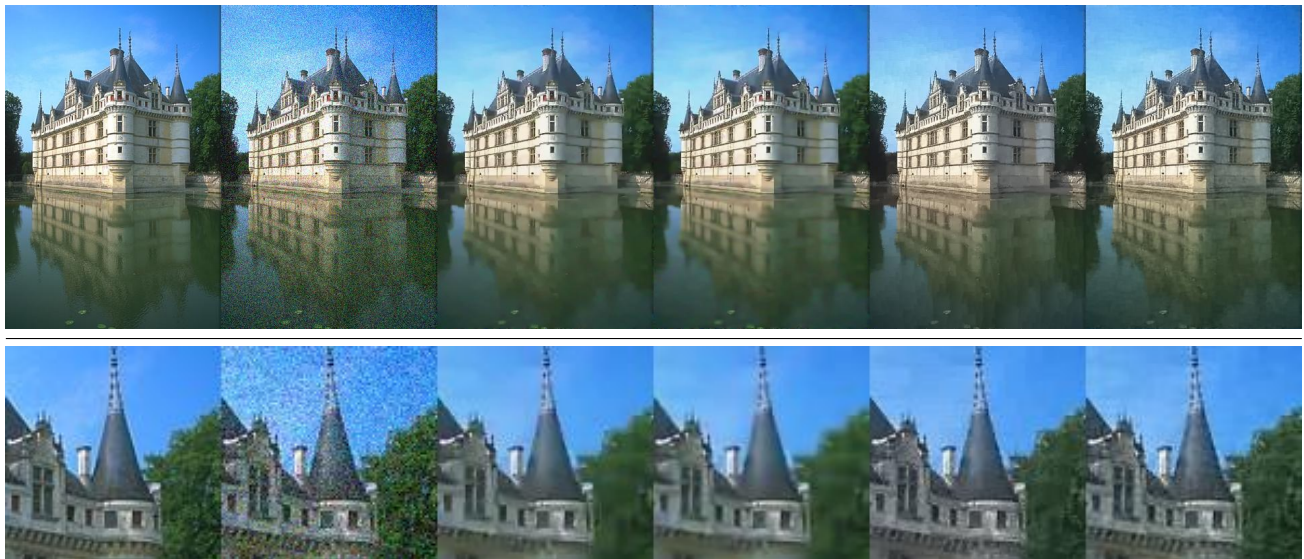
Figure 3. Top – from left to right: Original image, corrupt image with \sigma = 25 in all channels (PSNR = 20.46), denoised image using 3x3 model from Roth and Black (2005a) (PSNR = 29.91), using 5x5 model from Roth and Black (2005a) (PSNR = 29.82), using our 3x3 model (PSNR = 29.98), using our 5x5 model (PSNR = 30.41). Bottom – close-ups of all images.
