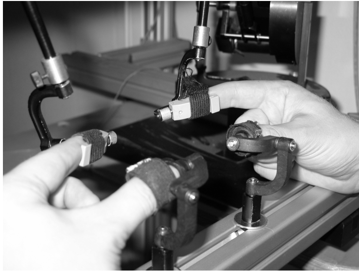
Fig. 1. Four-Finger PHANToM setup: The subjects' index fingers are put into one PHANToM force feedback roboter each, their thumbs are fixed in a gimbal on the bar in the front.
