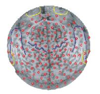
CTF whole-cortex MEG System **151 Channels 3 Localization Coils** Sampling rate: 312,5 HZ
