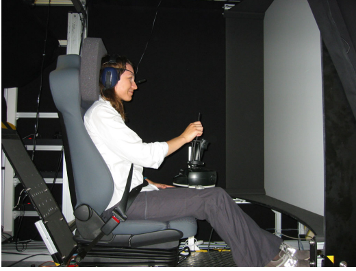
Figure 3: The experimental setup. Movement of the Stewart motion platform generates vestibular and somatosensory stimulation. Visual stimuli are generated by a projector mounted above and behind the observer. Both the projector and the screen are fixed to the platform and therefore fixed with respect to the observer.
