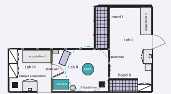
Figure 6a: Plan of three neighbouring NMR laboratories at ITT. Lab I: two accessible vented cabins (h = 3.30 m) for large scale devices, Lab II: NMR magnet, mobile vented cabin, Lab III: acquisition and probe preparation.
