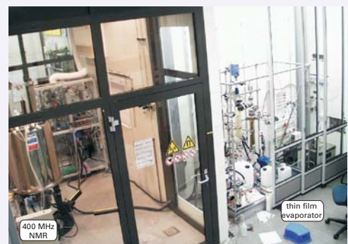
Figure 6b: NMR laboratory at ITT (University of Stuttgart): Direct coupling of thin film evaporator (right) with 400 MHz NMR spectrometer (left). For safety reasons both laboratories are separated by a transparent wall.
