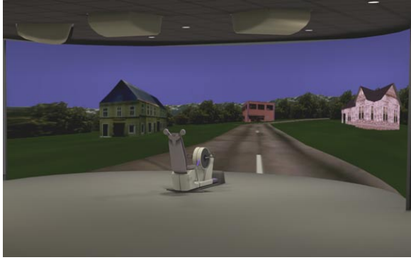
Figure 1: Virtual Environments Lab with 180° projection screen showing the Hexatown simulation. The subject was seated on a virtual reality bicycle in the center of the half cylinder.
