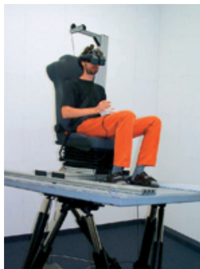
Fig. 1: Test subject on motion platform. The perception of intrinsic movement and sight are decoupled and manipulated separately. As a result, the researchers obtain feedback as to how the world is represented in the brain.
