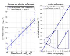
Figures 2 & 3: Typical distance reproduction and turn execution response from one subject. The left and right graph show the executed distance respectively turning angle, plotted versus their corresponding correct values. The blue enlargement in the right plot demonstrates the small within–subject variability for turns.
