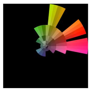
For the luminance histogram the luminance was averaged for all pixel within each segment. The number of pixels belonging to a segment does not contribute to the luminance histogram. The chart shows the mean luminances in each segment for the sample image.
