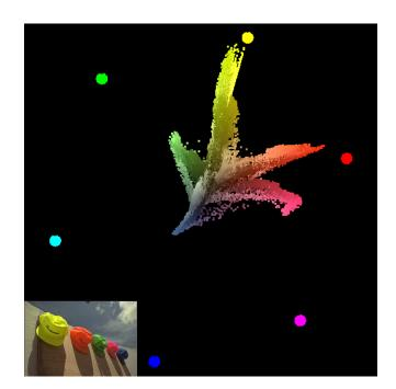
The outcome of the transformation process can be visualized by plotting the pixel colors according to their chromaticity coordinates in the color plane spanned by the color directions redgreen and yellow-blue (or hue and saturation in polar coordinates). The illustration shows the chromaticity distribution for the image with the hats at the bottom left. If more than one pixel had the same chromaticity, the luminance of these pixels was averaged.
