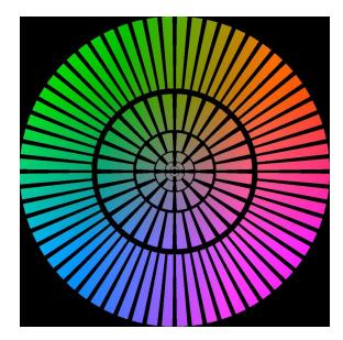
For indexing, the color circle was split into 127 segments. The categories were constructed so that the number of hue categories increased with increasing saturation. Six different rings were used for saturation, with the radius doubling as saturation increases. Thus, there is little discrimination of hues for unsaturated colors, whereas there are 64 different hues at the most saturated level.
