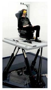
Figure 1: **The Stewart-Platform motion simulator.** The subject is seated blindfolded and with headphones on the platform. The platform is able to move in all 6DOFs independently.
