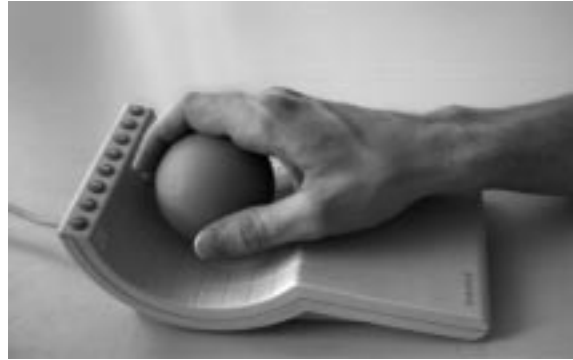
Figure 1: The “Spaceball” input device for rotation and translation of three-dimensional object models on a computer screen.
