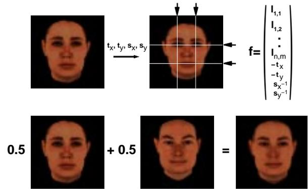
Figure 3: In this representation, the images are first aligned using two translations and two scaling operations. The image resulting from this alignment is coded together with the parameters describing the alignment. Although hardly visible in these small reproductions, the mean face still contains errors due to misalignment.
