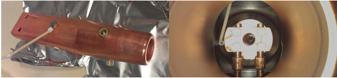
(a) Assembled collector. The electron beam enters the collector from the right.
