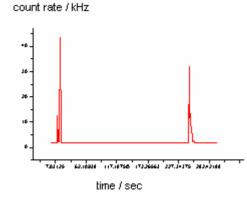
Figure4: Count rate of a 0.2 pM solution of QDs.
