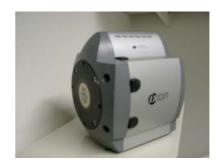
Figure 9: Andor's IXON DV 887 back-illuminated Electron Multiplying CCD-camera.
