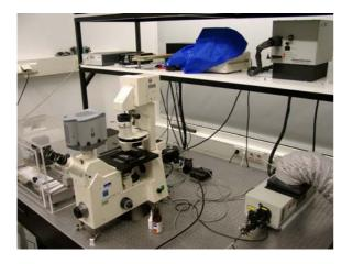
Figure 8: Overall setup of the EMCCD-coupled TIRF-microscope.
