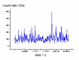
Figure 1: Fluorescence count rate of a 0.2 nM solution of quantum dots excited with 820 nm (average laser power 7.5 mW, emission < 700 nm).
