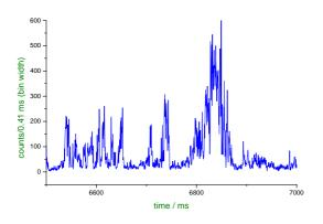
Figure 3: Multichannel scaler (MCS) trace of a 0.2 nM solution of QDs (bin width 0.41 ms).
