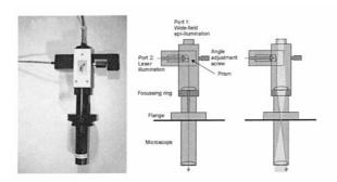
Figure 7: TILL-TIRF dual port epifluorescence condenser
