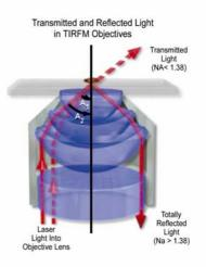
Figure 6: Radiation pathway within an objective-type TIRF-microscope
