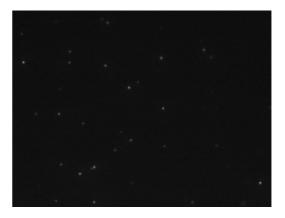
Figure 10a+b: Improved imaging conditions of the TIRF-microscope mode as compared to conventional bright field illumination using fluorescent beads of about 100 nm diameter.
