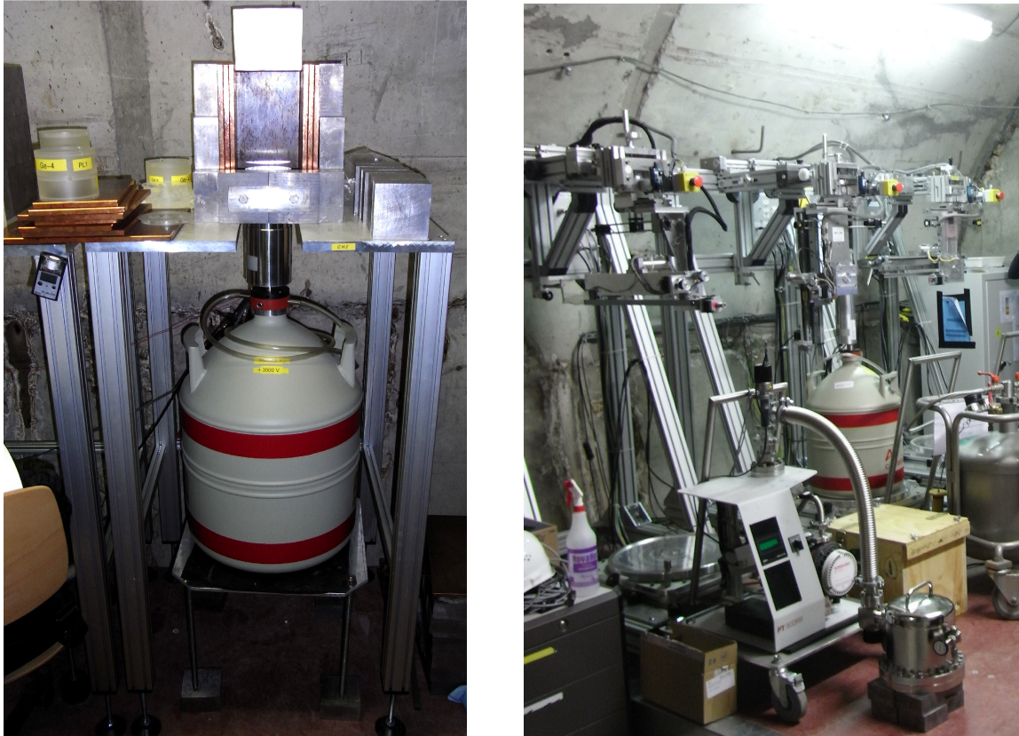
Figure 2. Left: One of two setups designed for static source measurements. Right: Three automated scanning tables for dynamic source measurements.
